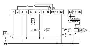
The CF3 enabling control deriving from the safety sequence (main controls device for safety such as thermostats, GAS min., Gas max., seal control, prewashing, etc....) shall be contacts without tension.
