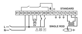
The **CF4** and enabling control deriving from the safety sequence (main controls device for safety such as thermostats, GAS min., Gas max., seal control, prewashing, etc....) shall be contacts without tension.
