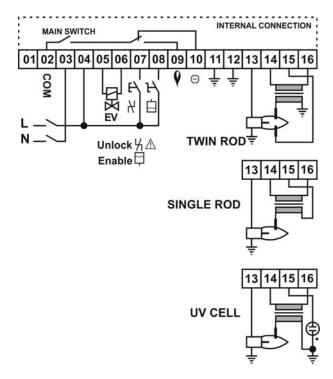
The enabling command of the CF5 that comes from the safety sequence (all the main control devices for safety purposes such as thermostats, GASmin, GASmax, leakage control, prewash, etc. ...) must be voltage-free contacts.
