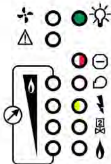
HT Transformer Not Connected Block
