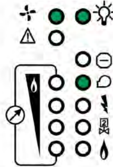
Enabled + Combustion Air Blower
