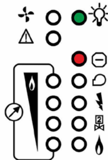
Burner Block Mode Flame Loss
